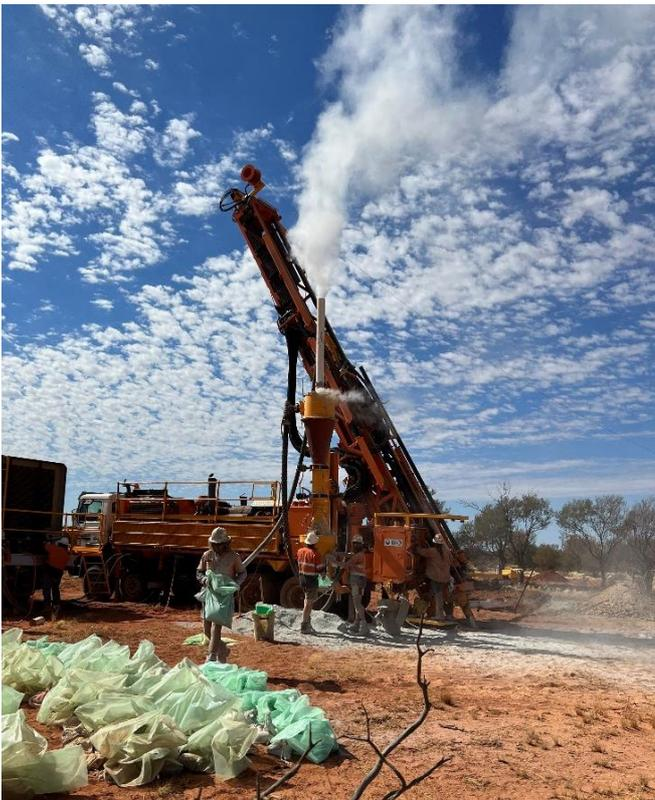
**Photo 1: RC Drilling rig onsite at Minos**
