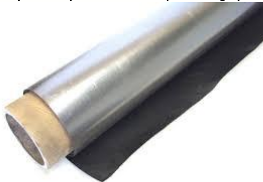
Figure 2: Graphite foil produced from expandable graphite
