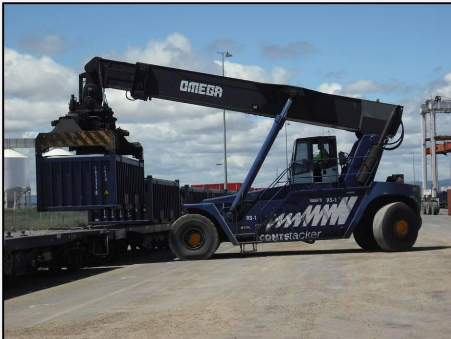
Figure 9: Reach Stacker Unloading Ore Container at Port Adelaide
