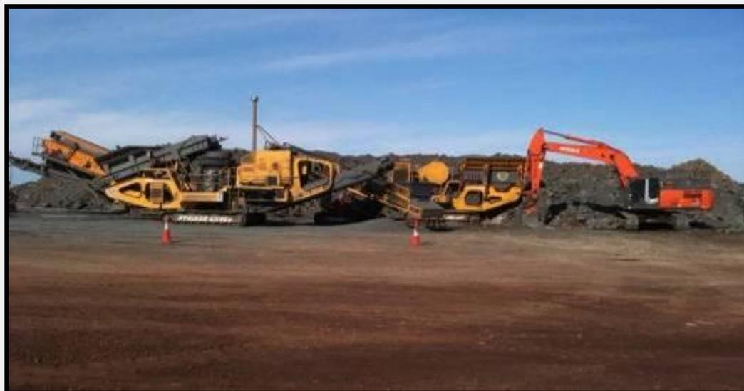
Figure 4: Exact Mining Services' mobile primary and secondary crushing units
