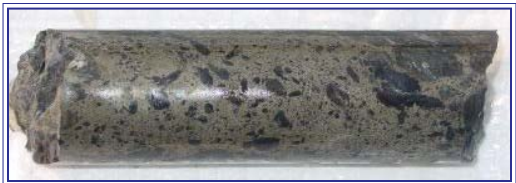
Photo 1 – Drill core from KPD101, 0.17m length from the massive nickel sulphide intersection.
