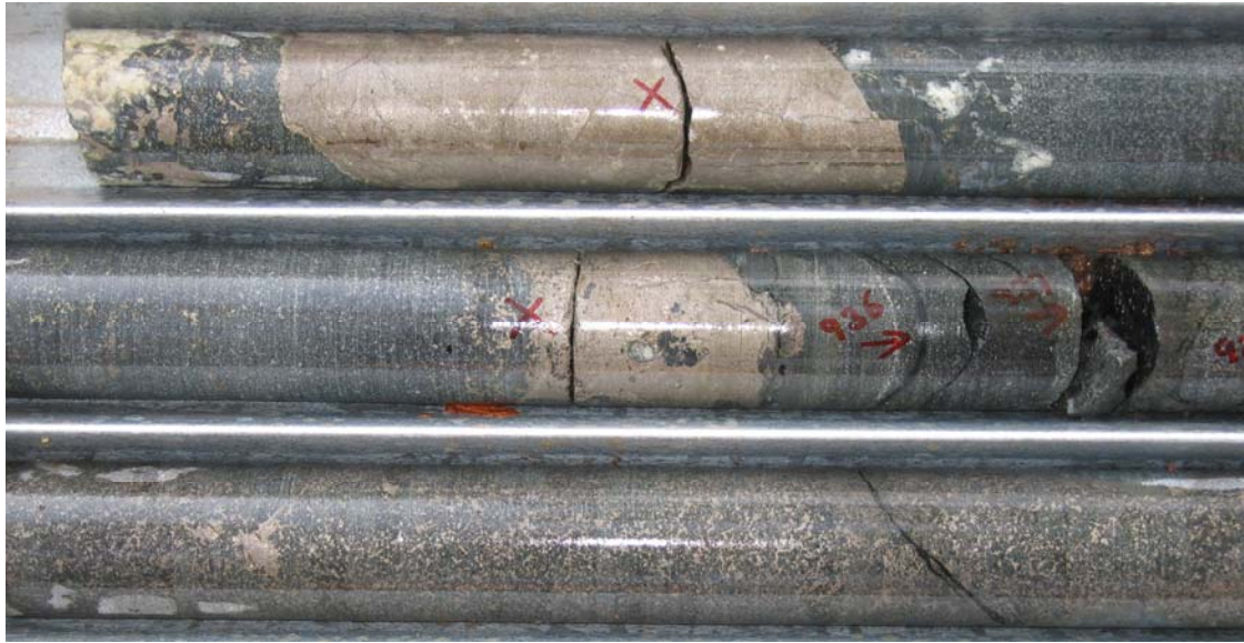
Photo 2: KPD122, Gabbro norite hosted massive, matrix & disseminated sulphide
