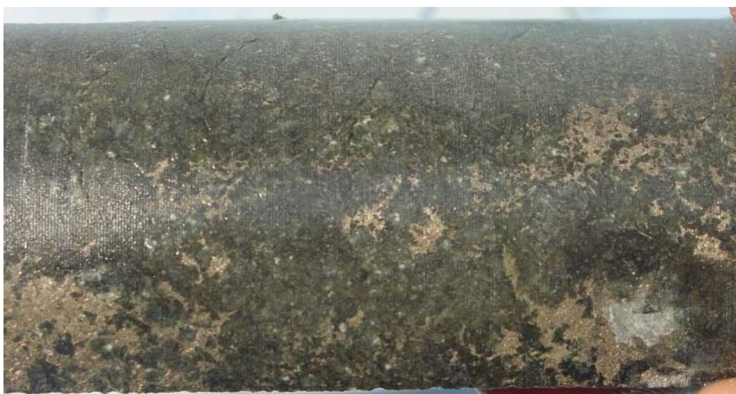
Photo 1: KPD112 - Gabbro norite hosted blebby & disseminated sulphide
