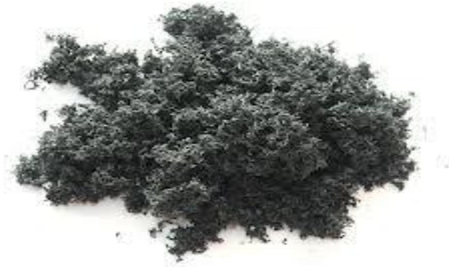
Expandable graphite is one of the fastest growing markets for graphite and has multiple uses, including the production of high-value graphite foils as shown below in Figure 2 (market price of ~US\$ 50,000/t) which are used as heat shields in electronic devices, graphite paper used in the manufacturing sector, heat shield gaskets and other products such as fire and thermal seals for machinery and electronic parts.
